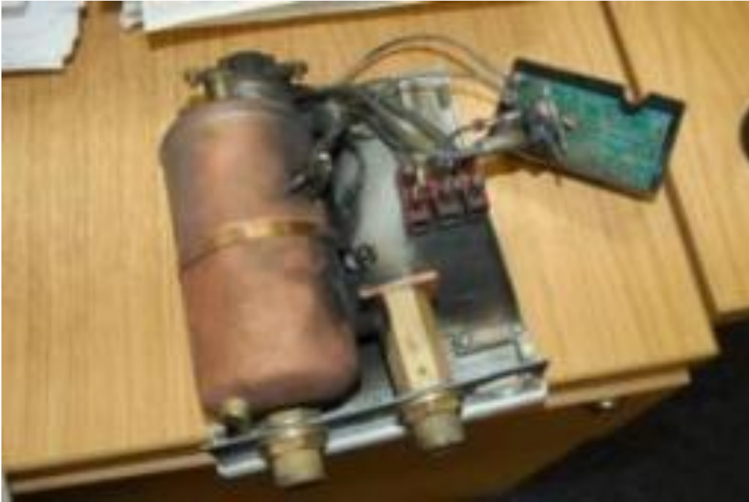
Sauna heater controller that caught fire due to counterfeit ICs
